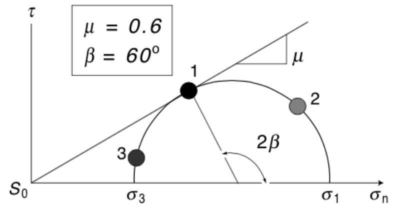
Optimal angle for frictional sliding:
