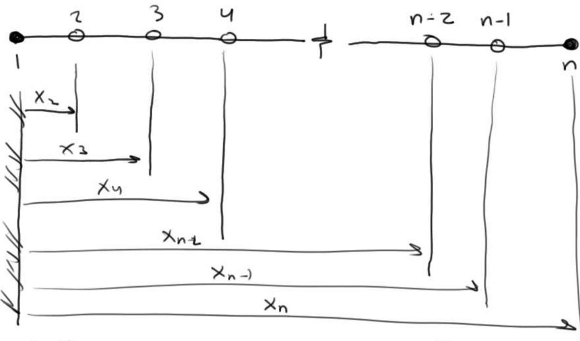
$$0 = \sum_{i=1}^{n-1} \left\{ \int_{x_i}^{x_{i+1}} \left[ a \frac{d\delta u}{dx} \frac{du}{dx} + \delta u u - \delta u f \right] dx - \left[ \delta u(x) a \frac{du}{dx} \right]_{x_i}^{x_{i+1}} \right\}$$
