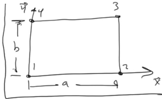
$$u_h(x,y) = c_1 + c_2 x + c_3 y + c_4 xy$$
