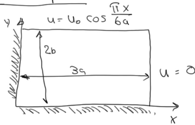
$$\begin{aligned} -k \nabla^2 u &= 0 \\ -k \left( \frac{\partial^2 u}{\partial x^2} + \frac{\partial^2 u}{\partial y^2} \right) &= 0 \end{aligned}$$
