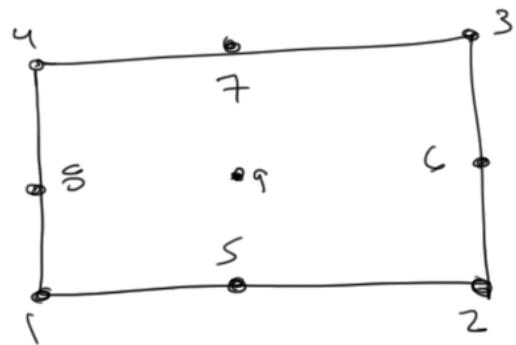
$$u_n(x, y) = c_1 + c_2 x + c_3 y + c_4 xy + c_5 x^2 + c_6 y^2 + c_7 xy^2 + c_8 x^2 y + c_9 x^2 y^2$$
