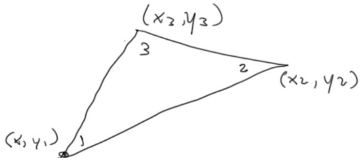
$$x(s,t) = x_1 + (x_2 - x_1) \frac{s}{a} + \left[ \left( \frac{c}{a} - 1 \right) x_1 - \frac{c}{a} x_2 + x_3 \right] \frac{t}{b}$$
