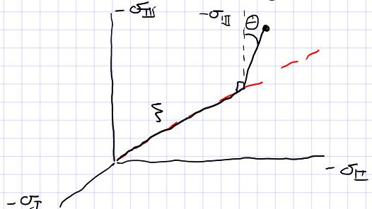
$\Theta$  is controlled by the relationship of the intermediate principle stress, i.e.  $\sigma_J$  to  $\sigma_I, \sigma_{II}$
